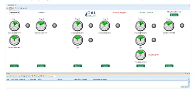
As a bath ages and gathers contaminants, the target conductivity in the bath will need to increase in order to keep the chemical concentration at its optimal level. The CALeye 2.0 uses titrations to calculate the new limits, and then auto-corrects itself to the new target range.
