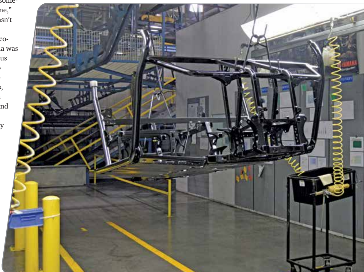
Yamaha's side-x-side utility vehicles get a powder coating following the new pretreatment system.
