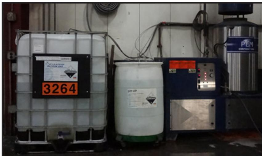
*CAM Superline’s High Pressure Pretreatment Setup includes a PEM Spray Wand Unit*
